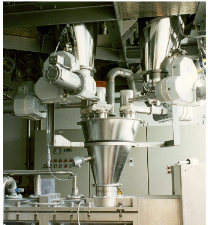
6. Multi-extrusion application with wood and resin, regrind, and additives on main twin screw extruder with flanking single screw extruders discharging to die head.
